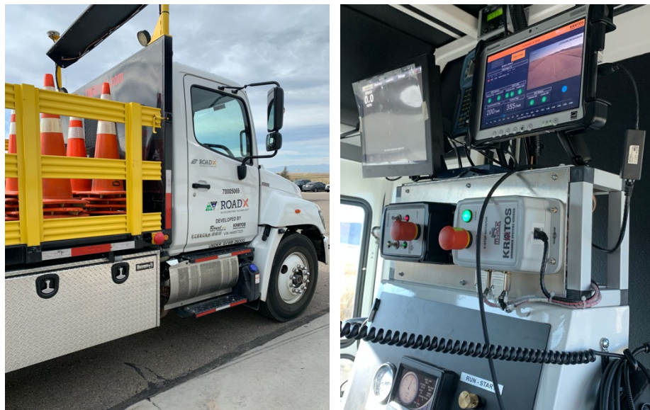
Figure 2. E-stop button outside of ATMA ( left ) and inside lead vehicle ( right )
