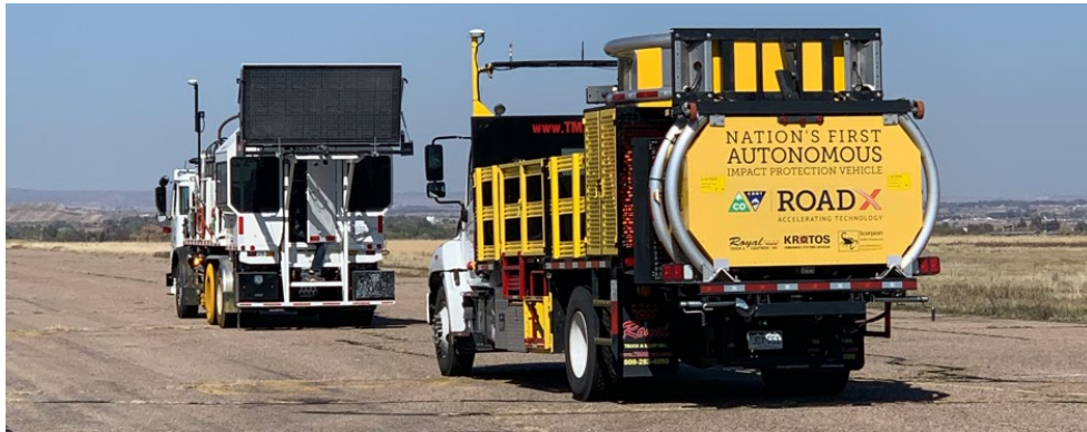
Figure 1. CDOT's lead vehicle ( left ) and ATMA follow vehicle ( right ).
